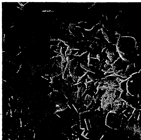
Figure 8.-Premier Chemicals MgO produced at Gabbs Nevada. SEM photomicrograph. MgO reacted in sealed vessel with \text{NaHCO}_3 at 90^\circ\text{C} for one week. Bottom of photomicrograph is 115 micrometers in length.
